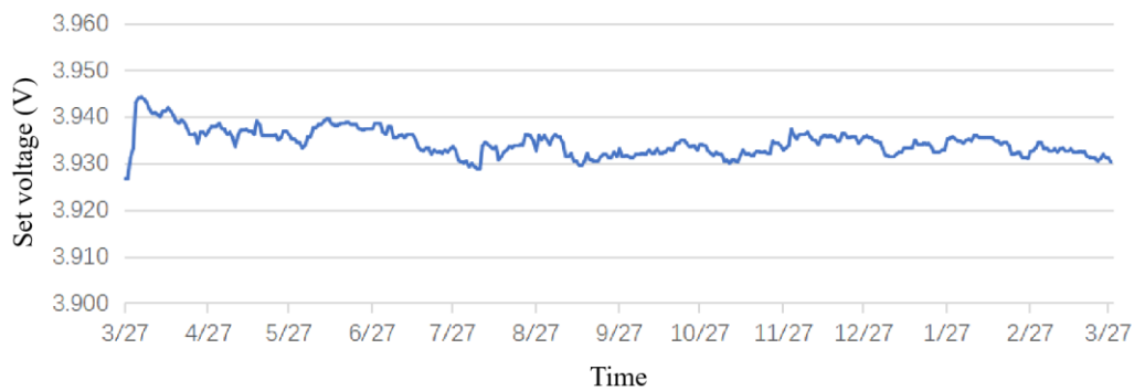
Figure 13. Set voltage curve during the monitoring period.
